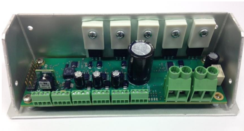
Image 1: The bi-directional SR-54 Series is a microcontroller based device with built-in monitoring and closed loop feedback control intelligence
