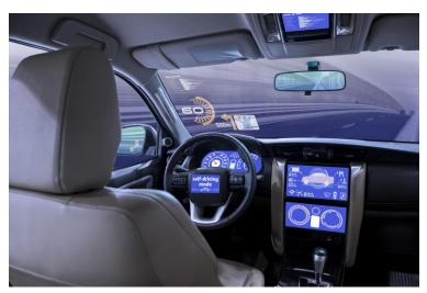
driving safely, OEM's are looking to keep the driver's eyes on the road by projecting information from the infotainment system onto the windshield. Additional safety features such as enhancing sign recognition to the windshield, or displaying a pedestrian crossing the street as a marker on the windshield, could be possible to aid in advanced driver-assistance systems (ADAS).
