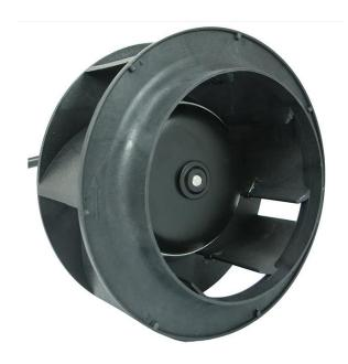
All of Orion Fans' AC and DC motorized impellers feature backward curved thermoplastic blades (metal blades are used on the largest AC models), a rugged diecast aluminum frame, and sealed dual ball bearings. Optional metal duct rings are available to fit all of the AC and DC motorized impellers. Custom packaging is available for most models upon request.
