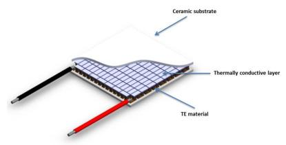
temperature differential of the critical device by as much as ~30°C from hot side temperature of heat exchanger. Heat will then need to be routed through a heat rejection mechanism, such as a heat sink and fan, to get the heat transferred into the air environment. It is critical that the hot side heat sink does not saturate otherwise heat will flow back into the device and heat it up. This is where TEM optimization for high coefficient of performance (COP) is critical.
