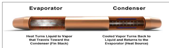
Figure 1: Heat pipe construction and principle of operation [1].
