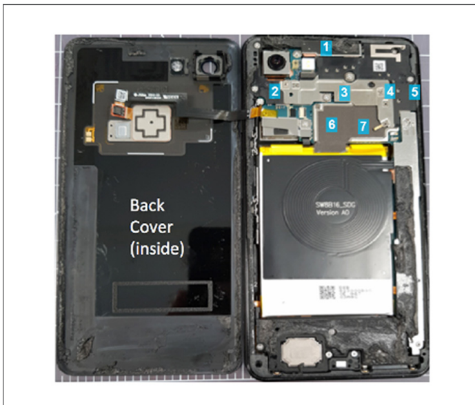
Figure 6: Google Pixel 3XL with back cover removed. Existing air gap thickness measured by conformable polymer at seven locations shown.
