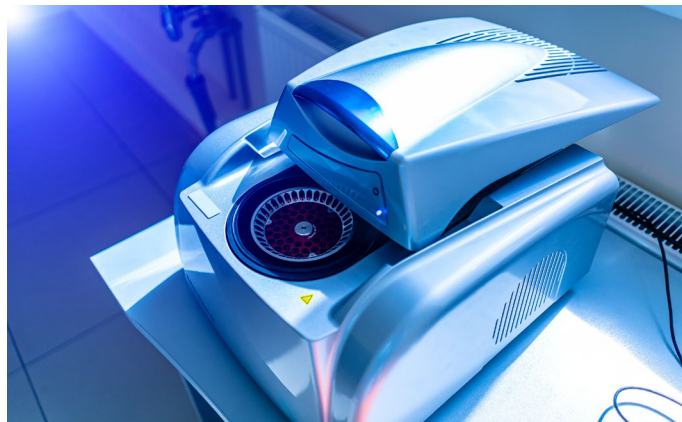
Modern thermocyclers utilize thermoelectric technology to deliver precise temperature control and fast ramp rates.
