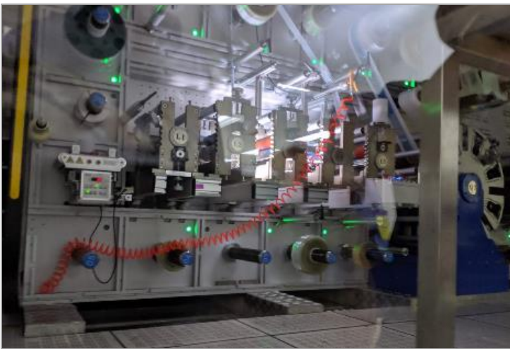
Advanced Rotary Die Cutting available globally in clean room environments.
