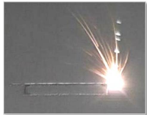
Fig. 1: An example of a titanium AM vapor chamber heat pipe being built vertically on a Renishaw AM 250
