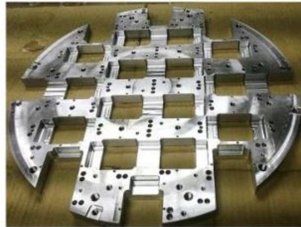
Fig 18: Complex Vacuum Brazed Liquid Cold Plate for Terrestrial Radio Telescope Applications
