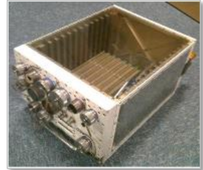
Fig 17: ATR electronics chassis with optimized vacuum brazed liquid cold plate sidewalls
