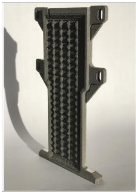
Fig 8: Titanium-Water Additive Manufactured Vapor Chamber Heat Pipe Capillary Wick Test Piece with Integrated Lattice Structure
