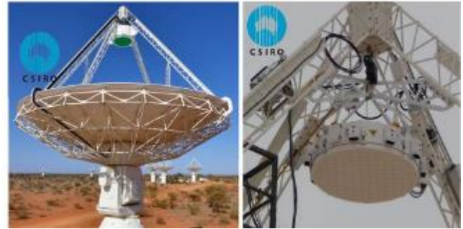
Fig 10: Photographs of an ASKAP radio-telescope with and close-up view of the PAF receiver module with integrated Aavid UK heat pipe receiver disc (CSIRO).
