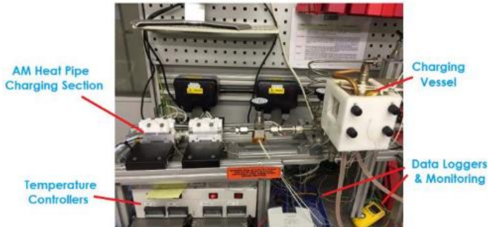
Fig.5: Lab-scale ammonia charging facility in the Boyd UK Design Center
