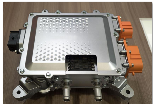
Example of an EV inverter – with cut out.
