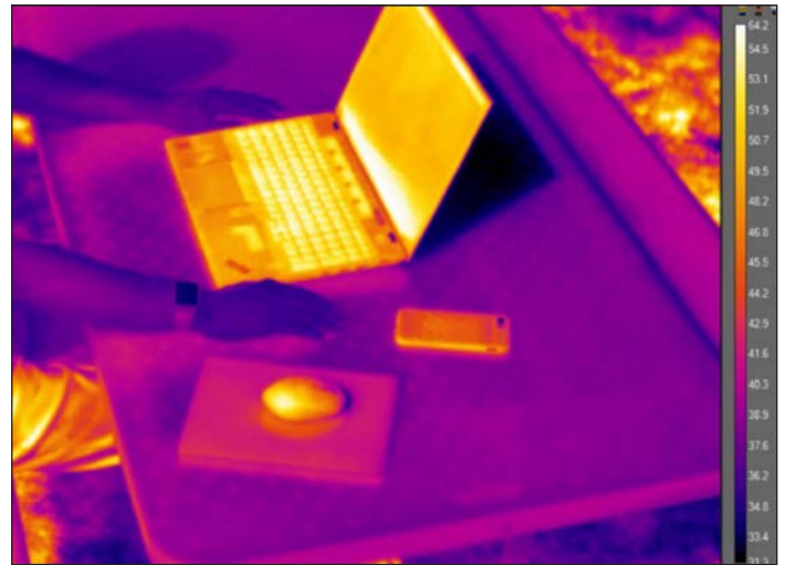
Figure 1: Infrared image of common consumer electronics during outdoor usage (°C)
