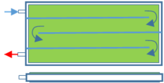
Fig. 2. Schematic of baseline battery cold plate showing top view (above) and side view (below) with flow baffles
