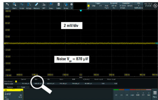
Noise is a function of vertical scaling. Choose the most sensitive vertical scale to reduce noise. In this example, 2 mV/div scales produces noise that is about 3 1/2 times smaller than noise at 20 mV/div.
