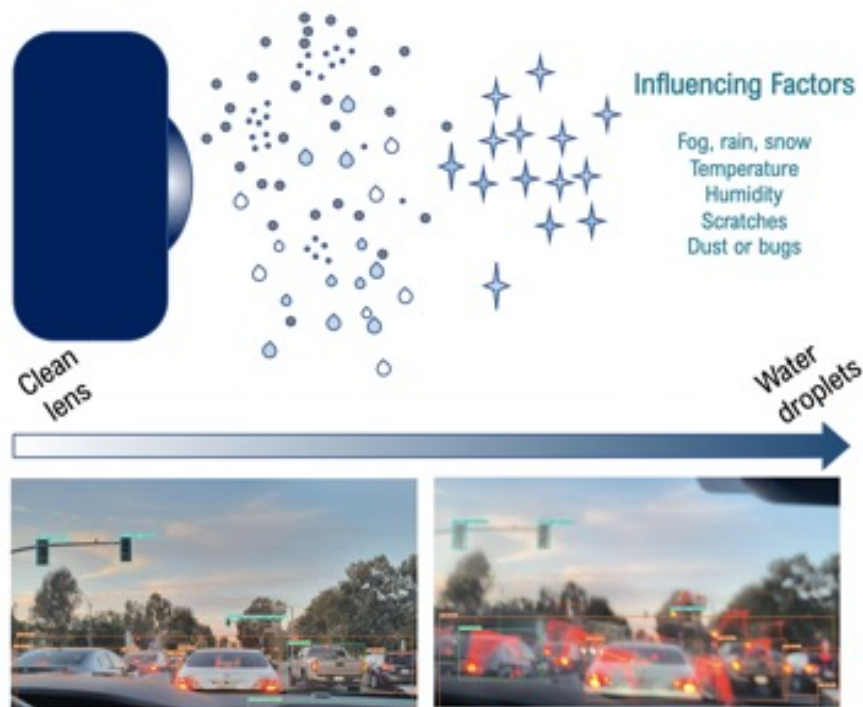
Figure 3 - Computer vision challenges and difficulties shown with declining classification count and accuracy when comparing images taken from a clear lens (left) to images from a droplet covered lens (right).
